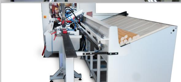
Outfeed discharging system with motorized conveyor belt, separator and pieces' collector/stacker
