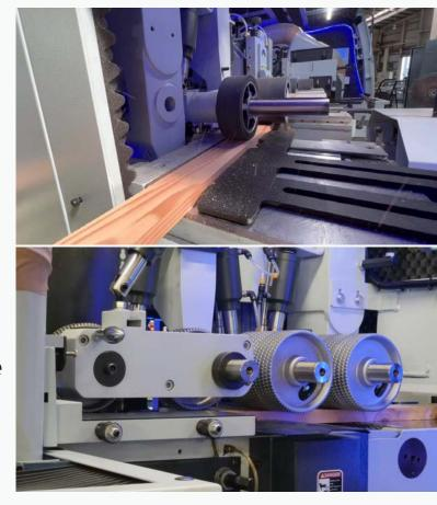
SURFACE PRE-WORKING MACHINE FOR EDGE GLUE MANUFACTURE
