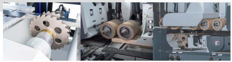
Using special milling spindle to produce the high-friction surface, making good quality and longer lifetime edge glue production.
