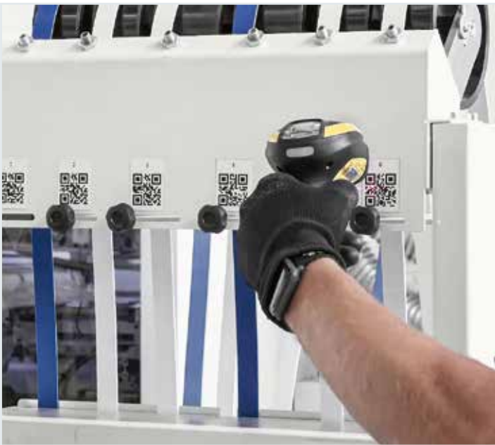
Edge store manager (opt.) A single database of all the customer’s edges, with rapid association of the machining program with the edge used, thanks to the “edge store manager” software. Coding with label and detailed report of the used and remaining edge.
