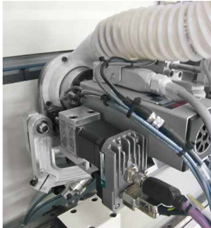
Excellent processing also with change of material or set-up thanks to the microadjustment system of the tool position by HMI. The tool is always in the right processing position.
