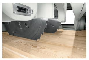
Double machining head unit for parallel operations and tool changes in masked time.
