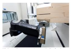
High performance electrospindle for heavy duty operations on all types of wood.
