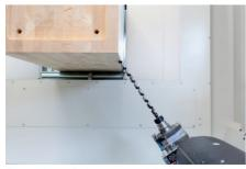
Execution of through or blind holes on all workpiece sides.
