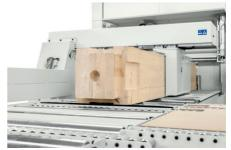
Automated handling of elements of up to 4 tons.
