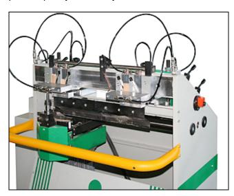
The machine has been designed to work eight pieces at a time (four male and four female joints in one work cycle). The particular characteristics of this machine, and the variable pitch program, let you work very small pieces (30 x 60 mm) for cigar boxes, jewellery boxes, or drawers with dovetail joints.
