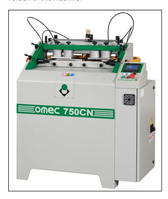
This model is equipped with a spindle unit and a milling cutter that can be used to manufacture
