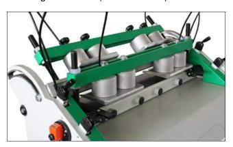
The machine, equipped with a 90° tilting workbench lets you produce drawers with curved and shaped front pieces.
