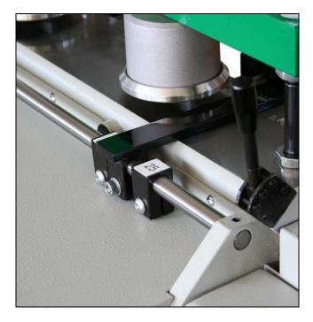
The CNC system also allows operators to move the position of joints on the work-piece by increasing or decreasing the distance of the first joint from the edge.
