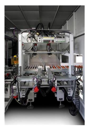
Automated single front head line sawing machine with electronic blade tilt angle control. It consists of:
