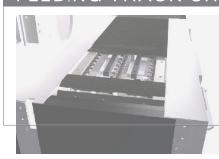
The feed belt runs along 2 hardened steel guides. The cast iron pad is fastened on a chain thus offering the following advantages:
