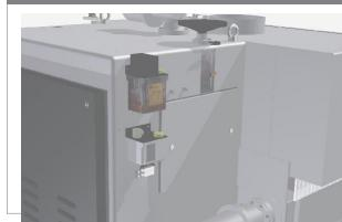
Machine lubrication is automatic . The oil distribution system supplies the single lubrification points in differential way at a pressure of 10 bar, thus ensuring maximum efficency also against risk of dogging. The oil flow rate is with a fully electronic regulation and has several setting.
