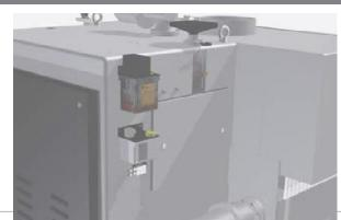
Machine lubrication is automatic. The oil distribution system supplies the single lubrification points in differential way at a pressure of 10 bar, thus ensuring maximum efficency also against risk of clogging. The oil flow rate is with a fully electronic regulation and has several setting
