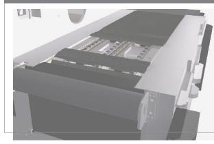
The feed belt runs along 3 hardened steel guides. The cast iron pad is fastened on a chain thus offering the following advantages:
