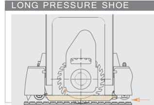
The long wooden shoe allows per-fect holding of the plank, even if warped in the blade compartment, thus preventing the blades from removing or splitting cracked or thin planks.
