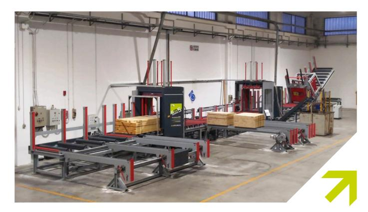
The system can be installed inside or outside the factory and can work with dried or frozen packs without any problem, cutting a 1300x1250mm (W x h) pack to the desired length in about a minute and a half. The best machine on the market for this type of work, produced since 1980, more than 700 have been delivered all over the world. The cutting line can be fully automated, allowing to reduce costs and increase precision and productivity.
