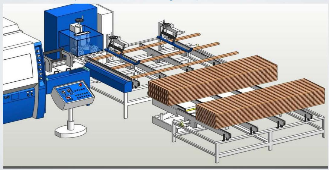
Auto. infeed chains move the stacked material to Hydro elevating platform that slow
