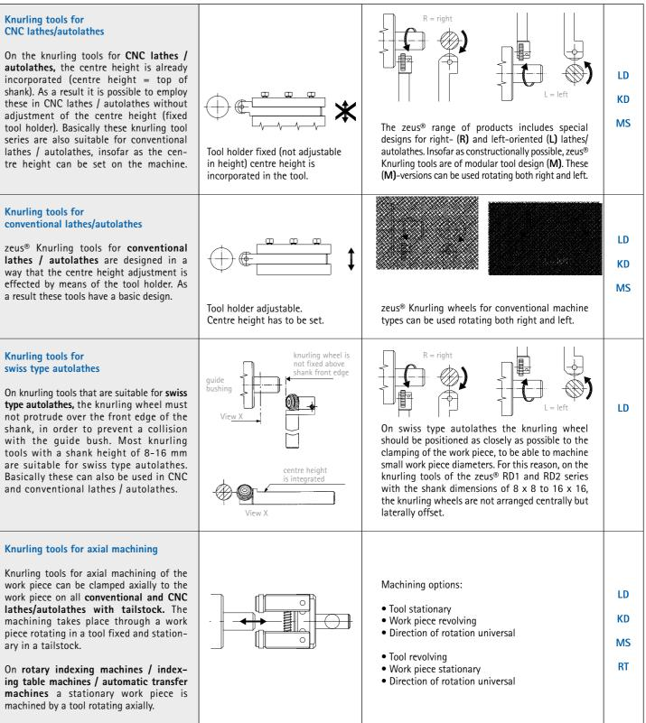
On rotary indexing machines / indexing table machines / automatic transfer machines a stationary work piece is machined by a tool rotating axially.
