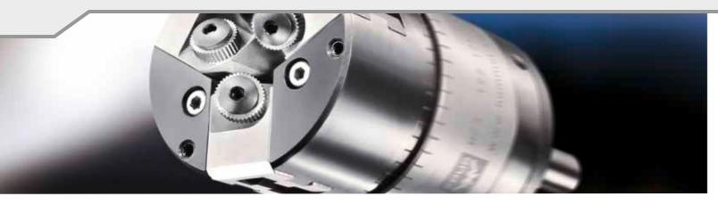
The zeus® RF3 series is designed for the fine machining of very small and thin-walled work pieces in axial tool direction. The product series is suitable for producing straight and RGE profiles with high demands on surface quality and dimensional accuracy. Due to the special design with three knurling wheels operating, the lateral pressure is reduced to a minimum. zeus® RF3: A specialist for knurling thin or pressure-sensitive parts, as for example spindles, tubes, or delicate bushings.
