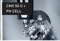
5-AXIS MILLING AND MODULAR AUTOMATION CONCEPT
