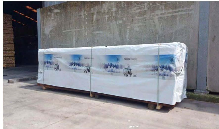
An even surface and a sufficient number of base battens.
