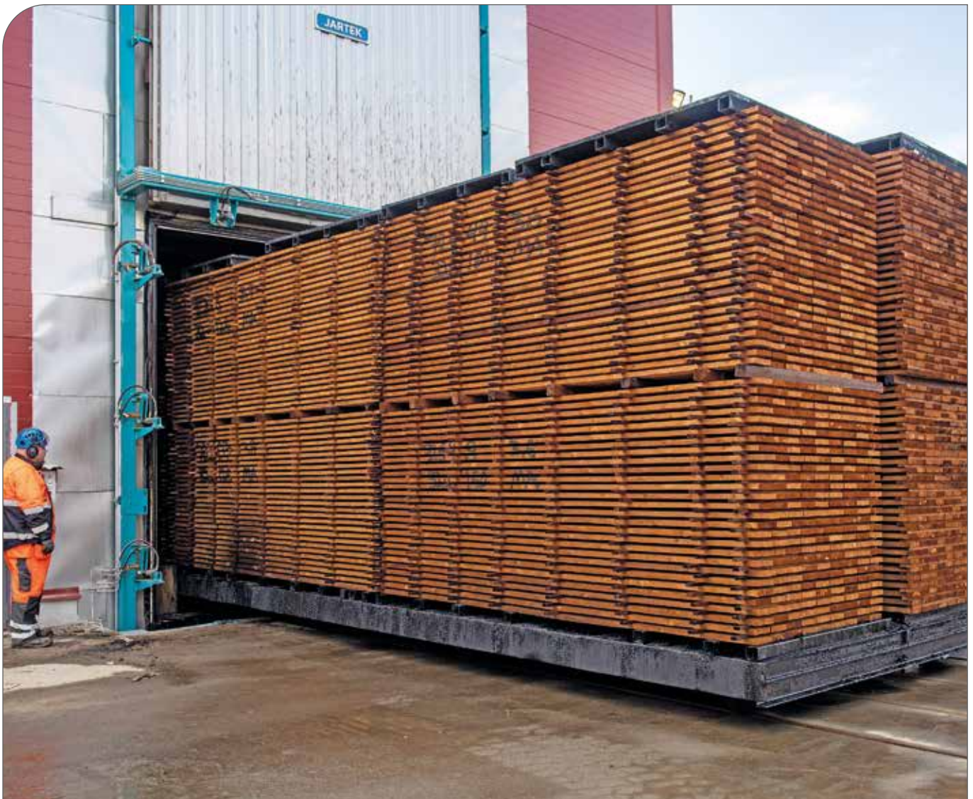
Figure 4. ThermoWood® being manufactured in process kiln.
