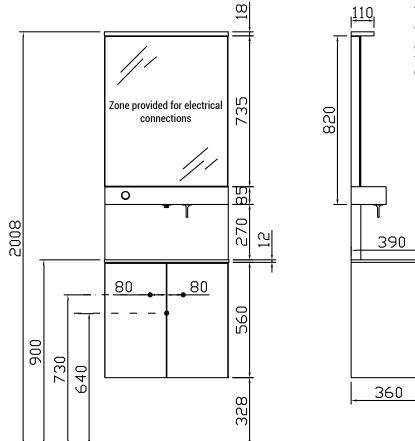
This type of washbasin is not fitted with an overflow.
